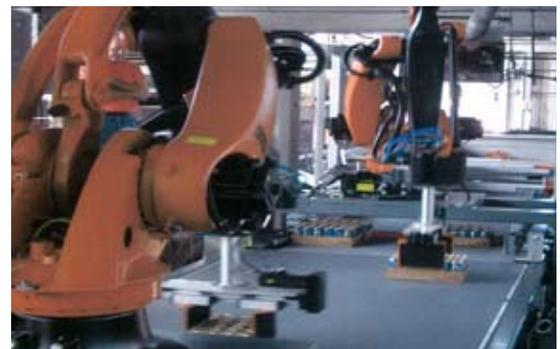
Robotic Case Turning and Positioning
