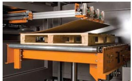
Sheet Placement on a Hydraulic Ram Hoist
